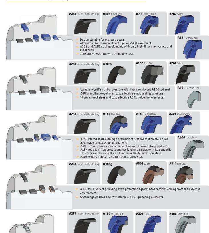
A406 static sealing element preventing well known O-Ring problems. A153 rod uring with high extrusion resistance at high pressures.
